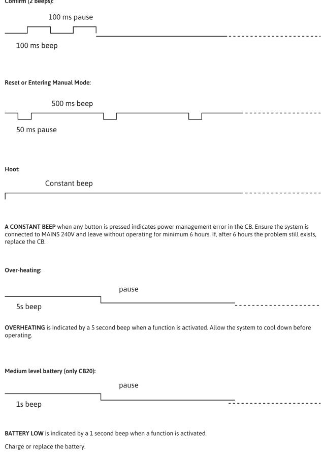
(If the temperature exceeds a pre-defined level the driving stops followed by a 5s beep tone. If the next activation is carried out before the temperature level is at an acceptable level, driving is not allowed and the 5s beep tone comes up).
