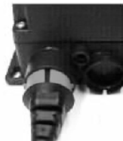
Mains cable on CB12 locked into position.
